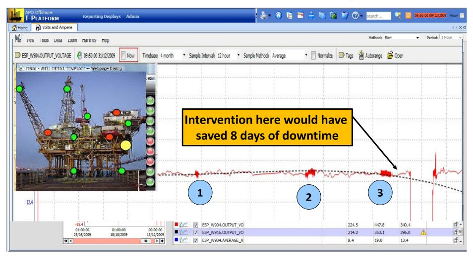
Pattern recognition by the neural network identified a complex series of events that did not exceed operator thresholds for current, temperature, or voltage, but when compared with a cubic trend line for two months before the event, were able to predict downtime in over 70% of failure cases in a given environment.
